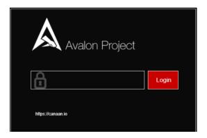
**STEP 4:** There is initially no password, so click Login to load the next interface. Once on the dashboard, click on Change Password to create a password.
