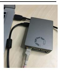
**STEP 2:** The default IP for the controller is 192.168.0.100. The IP address of the computer needs to be adjusted access to the controller.)
